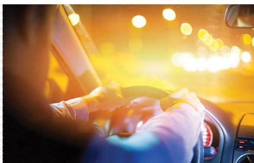
**4D COMPONENTS:** Flashing lights, point-like sources, high contrast of luminances, high blue component in LED headlights
