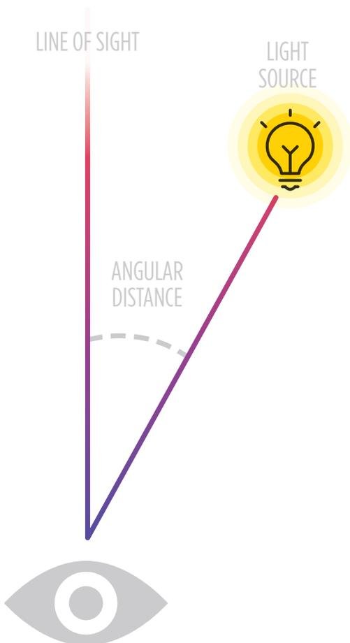
The spatial position of light sources and their size have a huge influence on the quantity and quality of light received by our eyes. In 1995 the CIE Technical Committee 3-13 developed a practical discomfort glare evaluation system for indoor lighting, which resulted in the Unified Glare Rating (UGR).<sup>16</sup>
